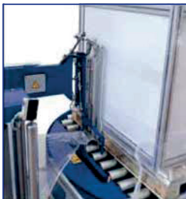
Cutting Unit: Binding film and cutting automatically.
